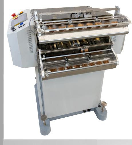
Equipped with two separate drive systems, it can alternately process two documents in a continuous strip independently, yet separately, merging them into a single trimming and crosscutting unit (CEM patent) to perform any interposition cycle under OMR/Barcode control.
